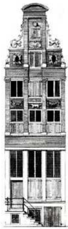
Figure 26 The complex composition of stairs and hatchway giving access to trading office, dwelling and rented out basement space.
